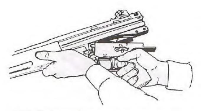
With the buttstock assembly removed, you can remove the entire trigger group by pulling downward on the pistol grip.
